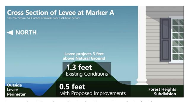
In proposed conditions, the ponding is reduced to a maximum depth of 0.5 feet.
