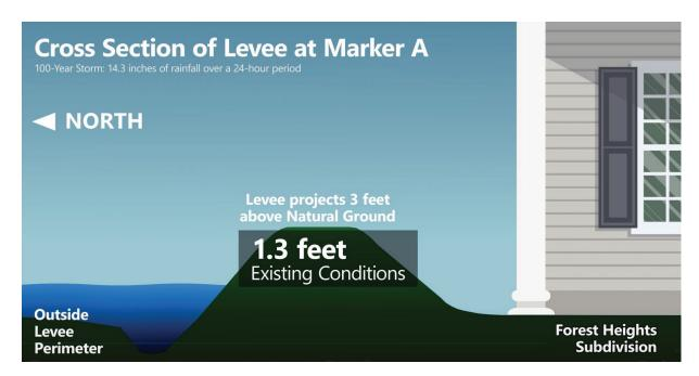
In existing conditions, water ponds up to a depth of 1.3 feet above the natural ground north of the levee.
