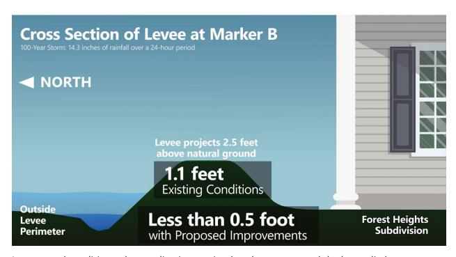
In proposed conditions, the ponding is contained to the area around the levee ditch.
