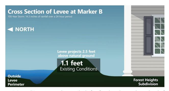
In existing conditions, water ponds up to a depth of 1.1 feet above the natural ground north of the levee.
