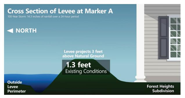
In existing conditions, water ponds up to a depth of 1.3 feet above the natural ground north of
