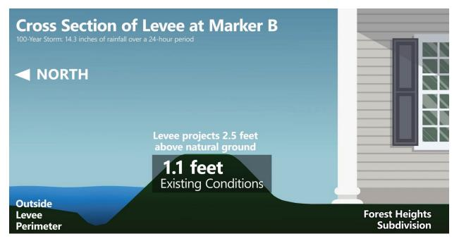
In existing conditions, water ponds up to a depth of 1.1 feet above the natural ground north of
