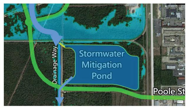
During a local rain event, storm water from the existing drainage way as well as the proposed roadway is diverted into the detention pond. During the rain event, stormwater is flowing into the pond at a higher rate than it is flowing out, causing the pond to fill and be released at a controlled rate.
