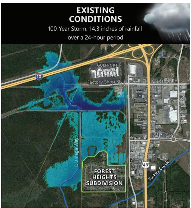
When it rains water from the surrounding areas enters the drainage way and the water level increases over time as shown on the left. A 100-year frequency storm event, which comprises 14.3 inches of rainfall over a 24-hour period, was used for this animation. This far exceeds the typical rainfall event.
