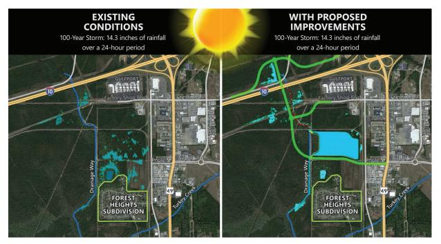
The detention pond continues to release the stormwater until after the runoff subsides and the pond reaches normal pool depth of 2 feet in 36 hours after the peak of the storm event.
