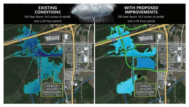
This detention pond provides storage volume for the storm water and helps reduce peak flows downstream of the pond.
