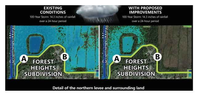
Here we can see a close-up of the northern portion of the Forest Heights neighborhood and levee during a 100-year 24-hour storm event. On the left side of the screen, today a significant amount of water drains to and around the northern Forest Heights levee. The water does not overtop the existing levee; however, there is potential for erosion of the levee over time.
