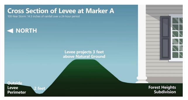
The animation shown here is a cross-sectional view of the northern Forest Heights neighborhood and existing levee at the location that was labeled "A" on the previous animation. In this location, the existing levee projects 3 feet above natural ground north of the levee and has a 2-foot-deep ditch which drains flow west around the levee. Note that this does not take the proposed Corps of Engineers levee project into account.
