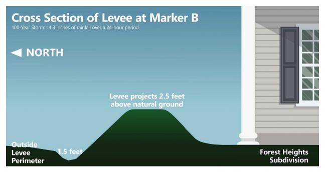
The animation shown here is a cross-sectional view of the northern Forest Heights neighborhood and existing levee at the location that was labeled "B" on the previous animation. In this location, the existing levee projects 2.5 feet above natural ground north of the levee and has a 1.5-footdeep ditch which drains flow west around the levee. Note that this does not take the Corps of Engineers proposed levee project into account.
