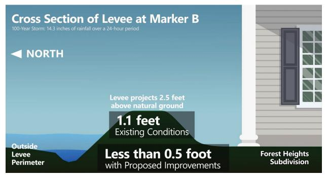
In proposed conditions, the ponding is contained to the area around the levee ditch.
