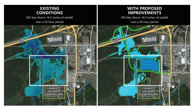
By routing most of the stormwater flow through the detention pond and through the existing drainage way, this greatly reduces water surface elevations upstream of the Forest Heights Subdivision reducing risk of potential flooding.
