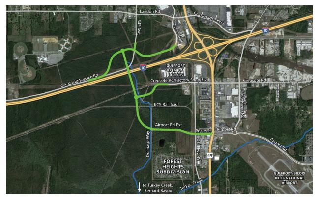
An existing drainage way flows under the interstate and railroad spur and continues south draining alongside the Forest Heights western levee and connects to Turkey Creek that drains east into Bernard Bayou
