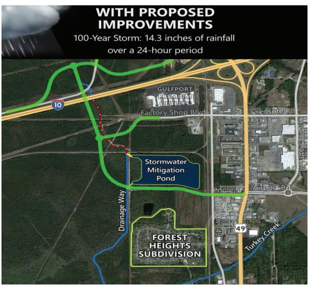
The water levels of a 100-year frequency storm event comprised of 14.3 inches of rainfall over a 24-hour period on the new roadway and stormwater system will be illustrated. This system includes a detention pond bordered by the railroad, the new roadway, and new roadside drainage. The pond will regulate the stormwater runoff into the drainage way.
