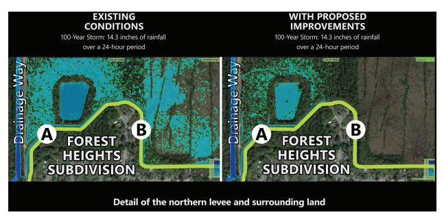
Note the location labeled A on the western end of the north levee and the location labeled B on the eastern end of the north levee. The following animation will show a comparison of the existing and proposed water surface elevations at these locations.
