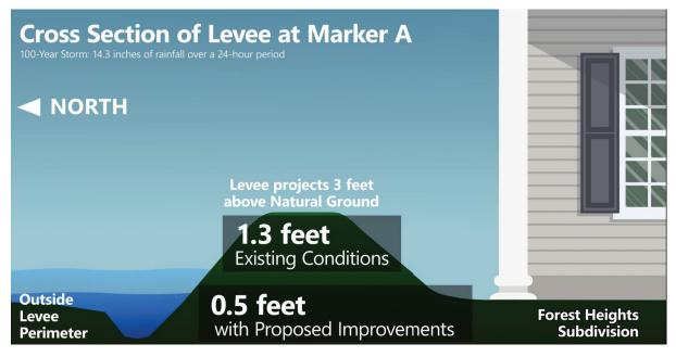
In proposed conditions, the ponding is reduced to a maximum depth of 0.5 feet.
